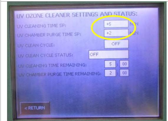
5. Set desired cleaning and purging time by pressing the white box to right of set point.
