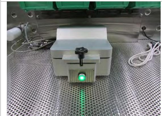
6. Press green button on front of UV ozone cleaner to start process. Button will illuminate.
