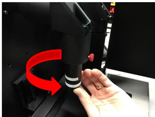
Figure 30: Attach reflectance optics.
