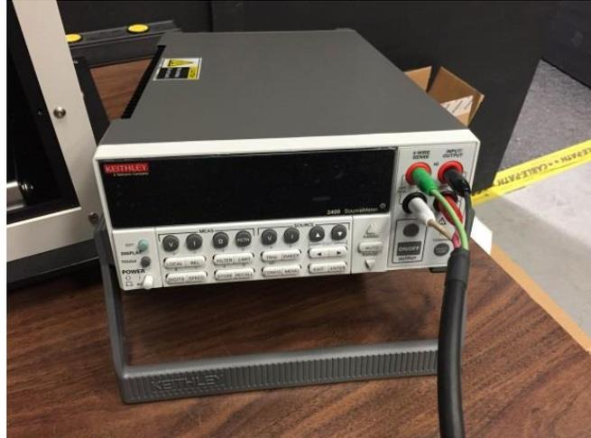
**Figure 40. Example of wiring to cell chuck and probe station, step 5 - Wiring between Keithley and SC-12 sample chamber.**
