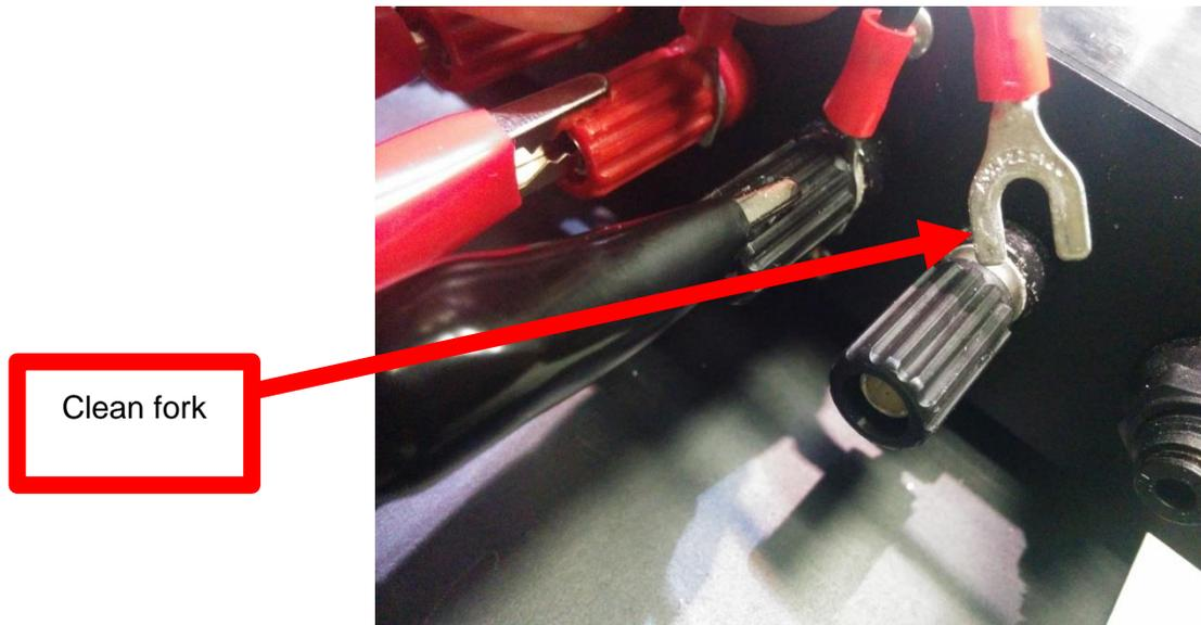
Figure 45. Electrical connection of probe station to cell chuck.
